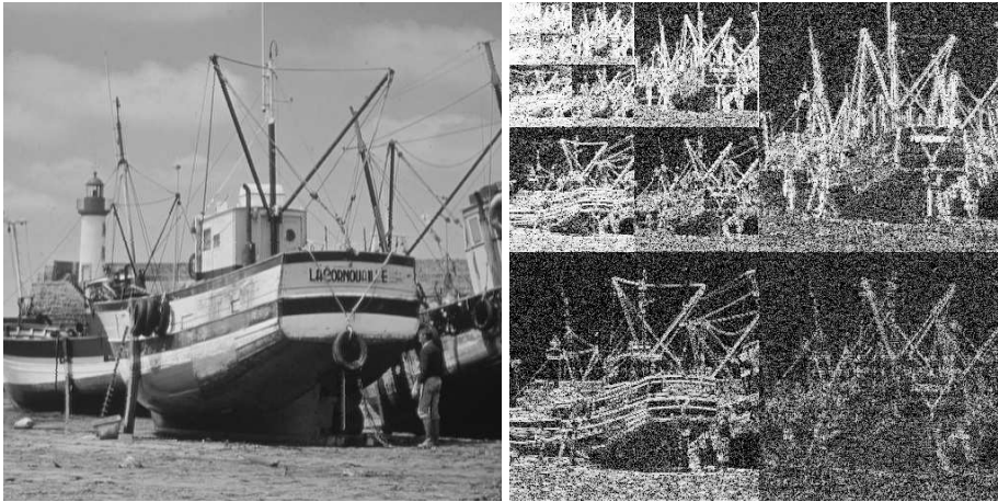
Figure 3: An example of the Daubechies wavelet transform. The original 512 \times 512 sized picture is on the left and its transform is presented with absolute values of the coefficients in logarithmic scale on the right.
